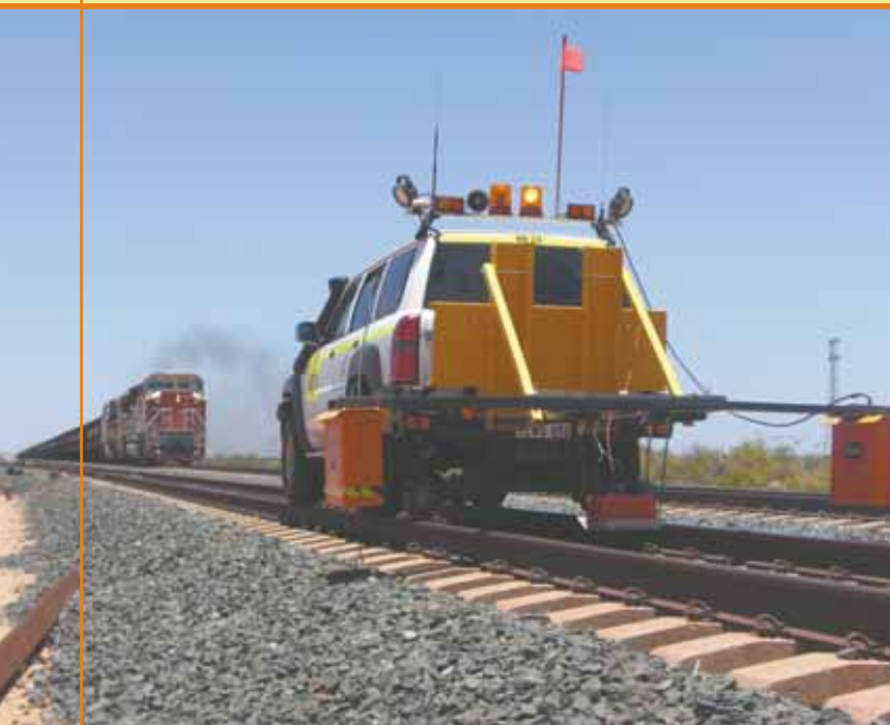
Trackbed investigations for maximising asset life, BHP Billiton Iron Ore, Western Australia.
